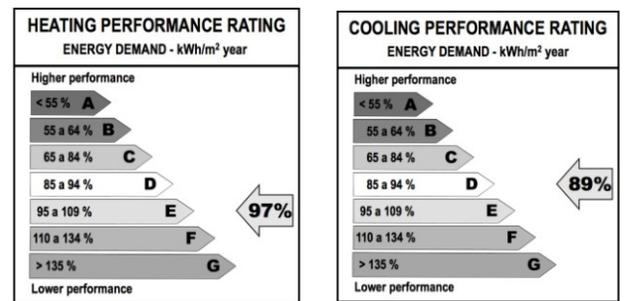
Figure 2: Building design energy rating according to the heating and cooling energy demand.
